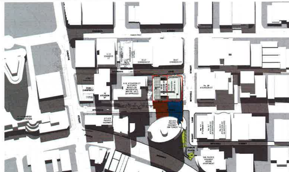
2 SHADOW DIAGRAM - 21st September, 1200AM 3503 SCALE 1:1000
