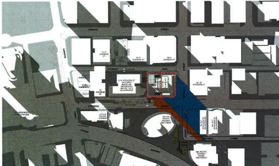
3 SHADOW DIAGRAM - 21st June 1600PM SCALE 1:1000
